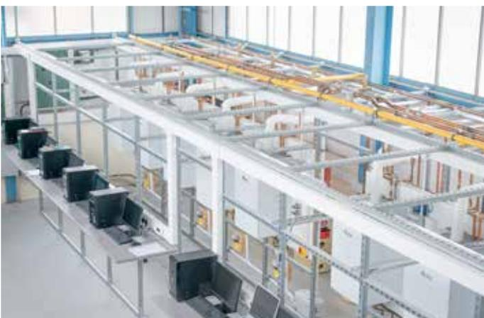
We have upgraded our boiler test centre in Unit 12 at Capenhurst to operate at full capacity, with 10 Flow boilers working continuously. These boilers are constantly monitored, generating useful reliability and performance data. Unit 12 is a stone's throw from the R&D workshop where the Flow boiler was developed and where future versions will be designed. Both facilities offer an impressive illustration of the scale and scope of the Flow operation.
